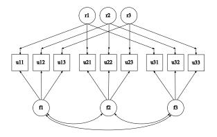
With categorical outcomes, ML estimation leads to numerical integration that is difficult with many dimensions/factors. The two-tier algorithm reduces the 6 dimensions of integration to 4. Bi-factor CFA has a similar structure that benefits from two-tier computing.
